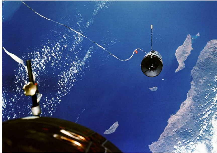
Figure 6.4.2-1. Gemini XI Spacecraft tethered to an Agena Rocket Casing on September 14, 1966 (Gemini XI command pilot Charles “Pete” Conrad and pilot Dick Gordon maneuvered the craft to keep the tether taut between the two; by firing the side thrusters to slowly rotate the combined spacecraft, they were able to use centrifugal force to generate about 1.5 \times 10^{-4} g of AG for about 4 hours; Image credit: NASA)
