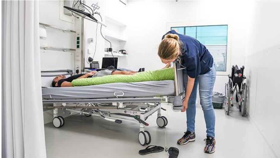
Figure 6.4.1-3. AGBRESA Participants' Beds tilted 6 degrees downward at Head End to allow Negative Effects of Weightlessness in Space to be induced on Earth [Braun 2019]
